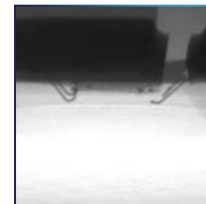
LED gold wire crack
